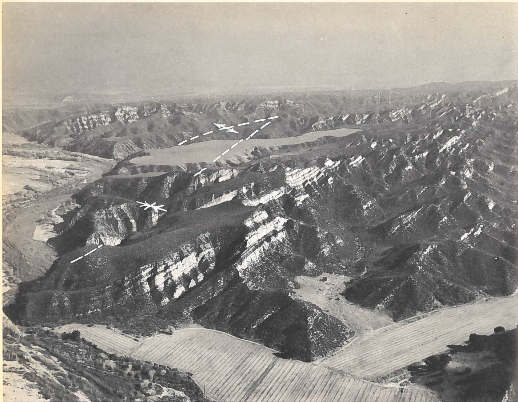
FIGURE 10. Typical exposures of the Saugus formation in the eastern Ventura basin, about 7 miles west of Saugus. These nonmarine strata, of late Pliocene and early Pleistocene age, are here broadly folded. Axial traces of two folds are shown by the dashed lines. Pacific Air Industries photo.
