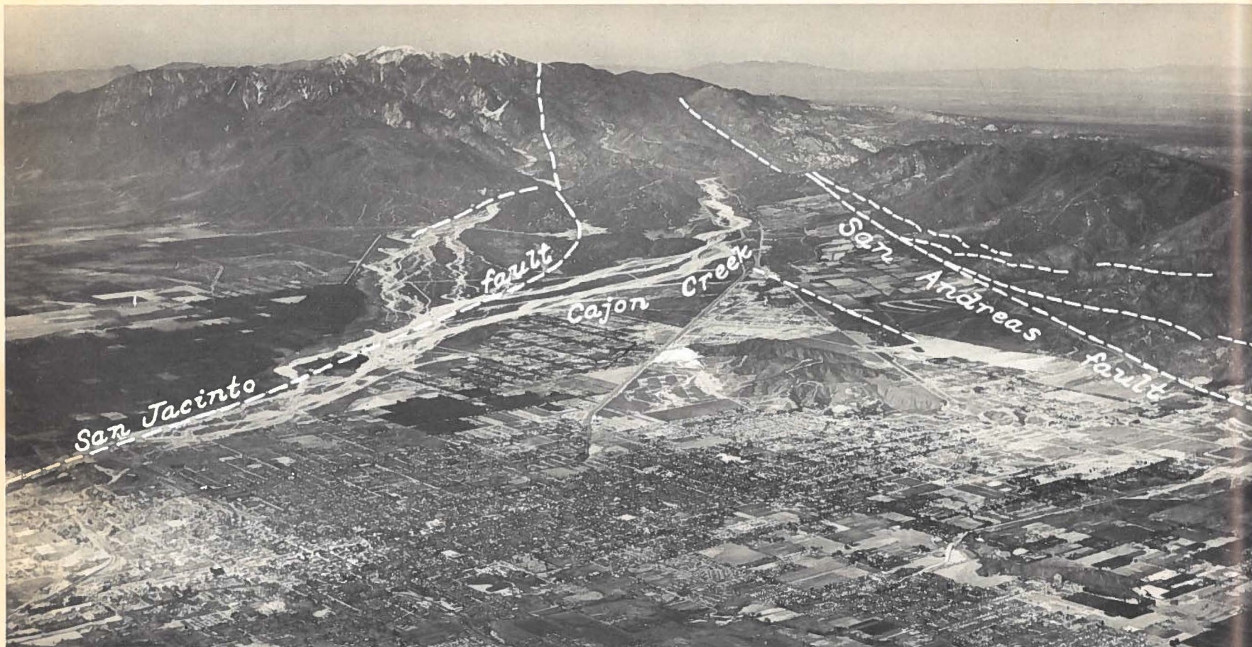
FIGURE 3. View northwest over San Bernardino, showing the San Gabriel Mountains (left) and San Bernardino Mountains (right). San Antonio peak is on skyline at left, and Mojave Desert is in distance at right. Light-colored outcrops in upper drainage of Cajon Creek beyond the trace of the San Andreas fault are terrestrial strata of Miocene age (see fig. 7). Traces of major faults are shown by dashed lines. Pacific Air Industries photo.
