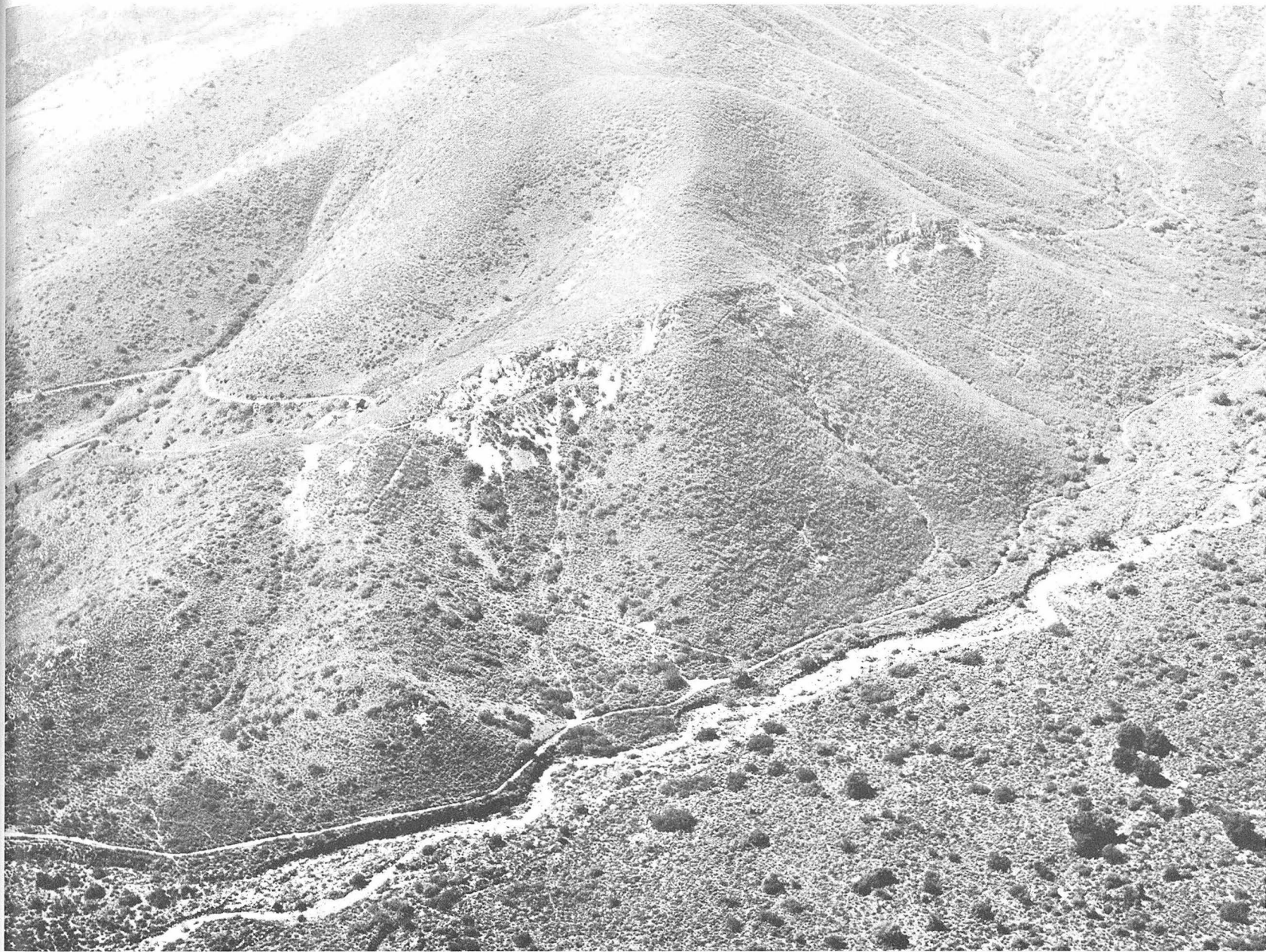
FIGURE 14. Northwestward aerial view of a part of Queen Mountain, Pala district, showing open cuts of the Stewart lepidolite mine. These workings are in the thick and bulbous southern end of a pegmatite dike that dips away from the observer, and they lead to tunnels and stopes that underlie much of the hill slope beyond the crest of the foreground ridge. The dike splits northward into two or more juxtaposed dikes whose outcrops are visible on the brush-covered slopes. Workings of the Gem Star mine appear below the cliffs in the right-hand part of the view. Pacific Air Industries photo.
