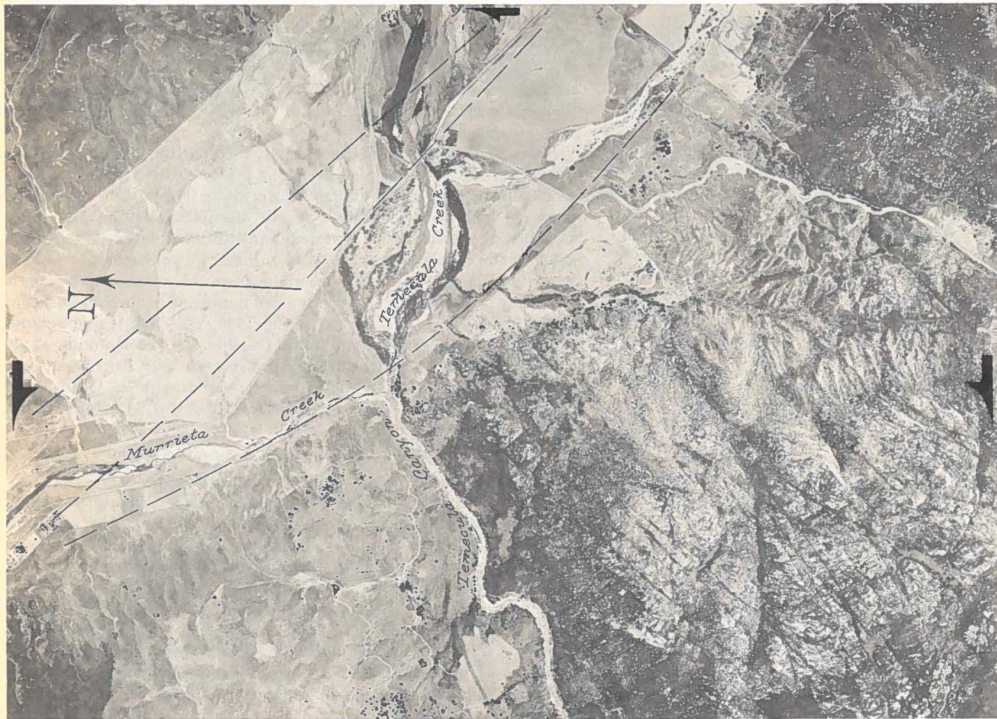
FIGURE 6. Vertical view of the area immediately south of Temecula, showing typical contrasts in weathering of different rocks. Jointed granodiorite forms rough slopes in south part of area, metamorphic rocks of Triassic age underlie the smoother slopes west of Murrieta Creek and north of the steep-walled Temecula Canyon, and arkose of Pleistocene age underlies the remainder of the area. Note the possible offset of Temecula Creek along the trace of one break (dashed line) in the Eisnorre fault zone. U. S. Department of Agriculture photo.
