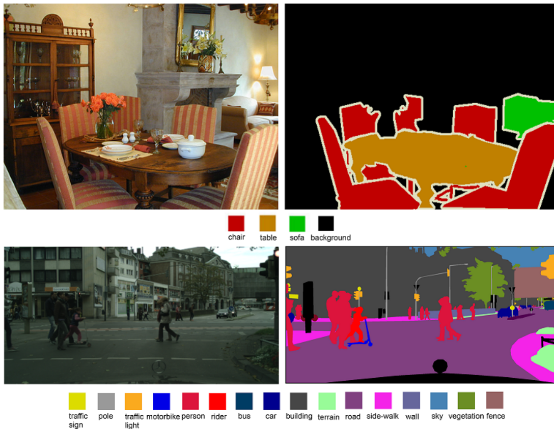
Figure 1.1: Semantic scene segmentation has many applications, such as in indoor scenes for human-robot interaction or in outdoor scenes for autonomous navigation.
