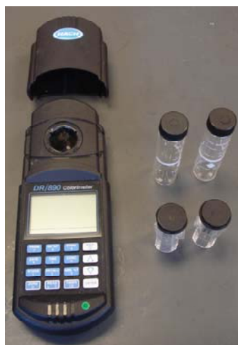
Figure 3.24. HACH DR/890 colorimeter.
