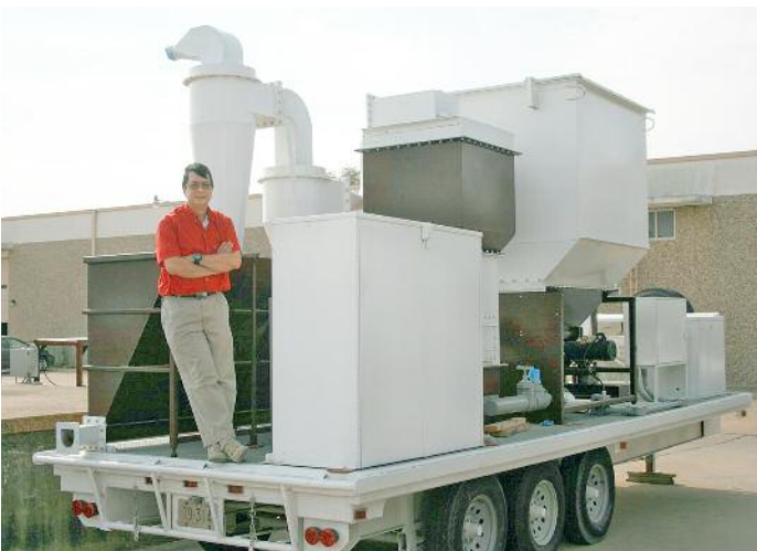
A mobile pyrolysis unit developed at Texas A&M University. Photo courtesy of Sergio Capareda, Texas A&M University.
