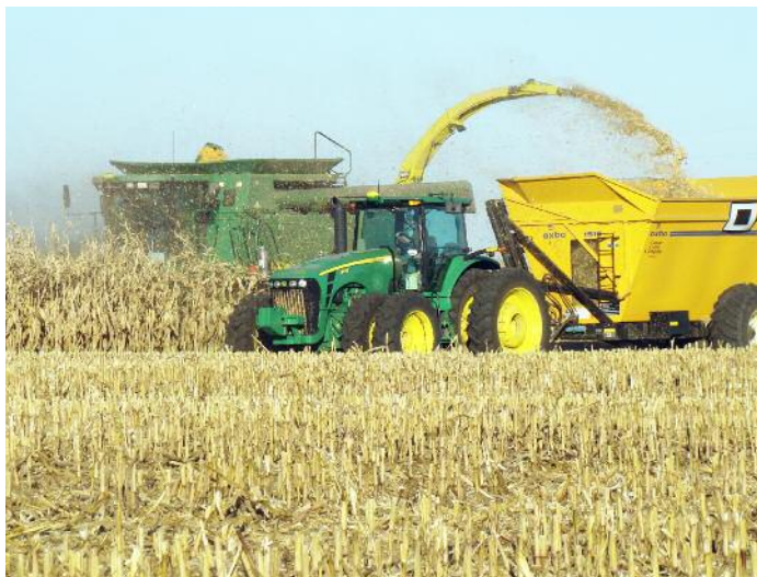
One-pass harvest of corn grain and stover in Iowa. Photo courtesy of Doug Karlen, USDA ARS.
