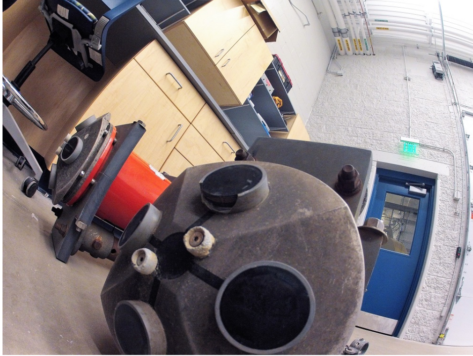
Figure 5.8: Damage to the ADCP transducer housing that was installed at the bow of the turbine deployment platform
