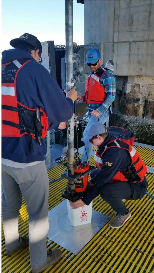
Figure A.2: ADCP rotation for calibration on 9/29/17
