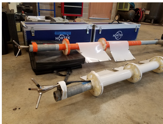
Figure 4.12: Final fairing design using 1/16 in thick HDPE sheeting and hose donuts
