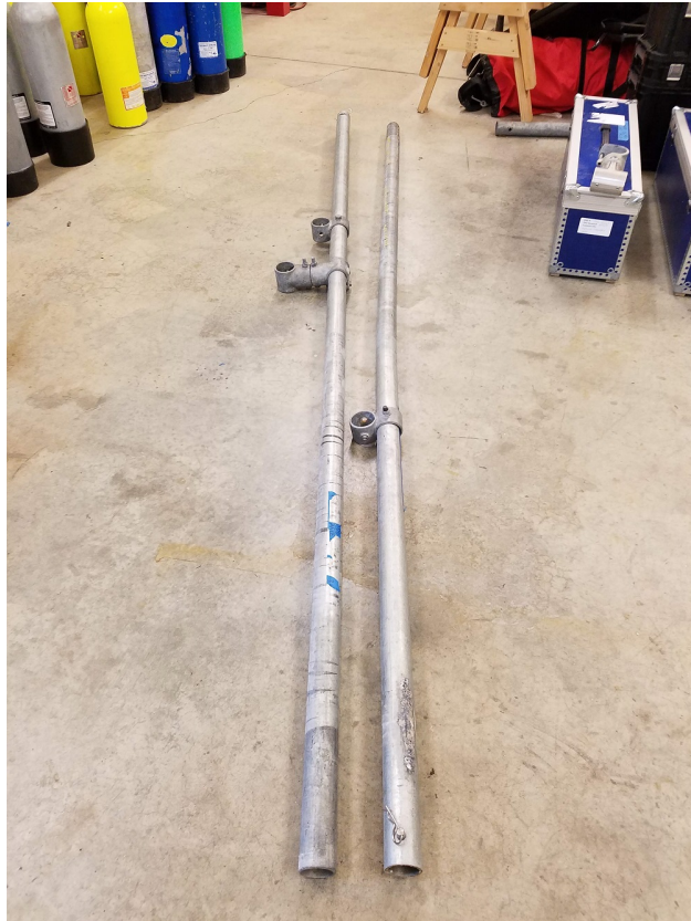
Figure 5.7: Bend in the mounting pipe (right) caused by the impact that caused damage to the ADV probe head on 2/4/19
