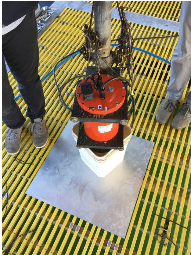
Figure A.1: ADCP set up for calibration on 9/29/17
