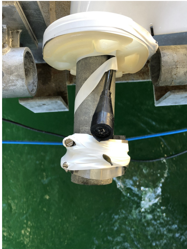
Figure 5.6: Damage to the ADV probe head on 2/4/19
