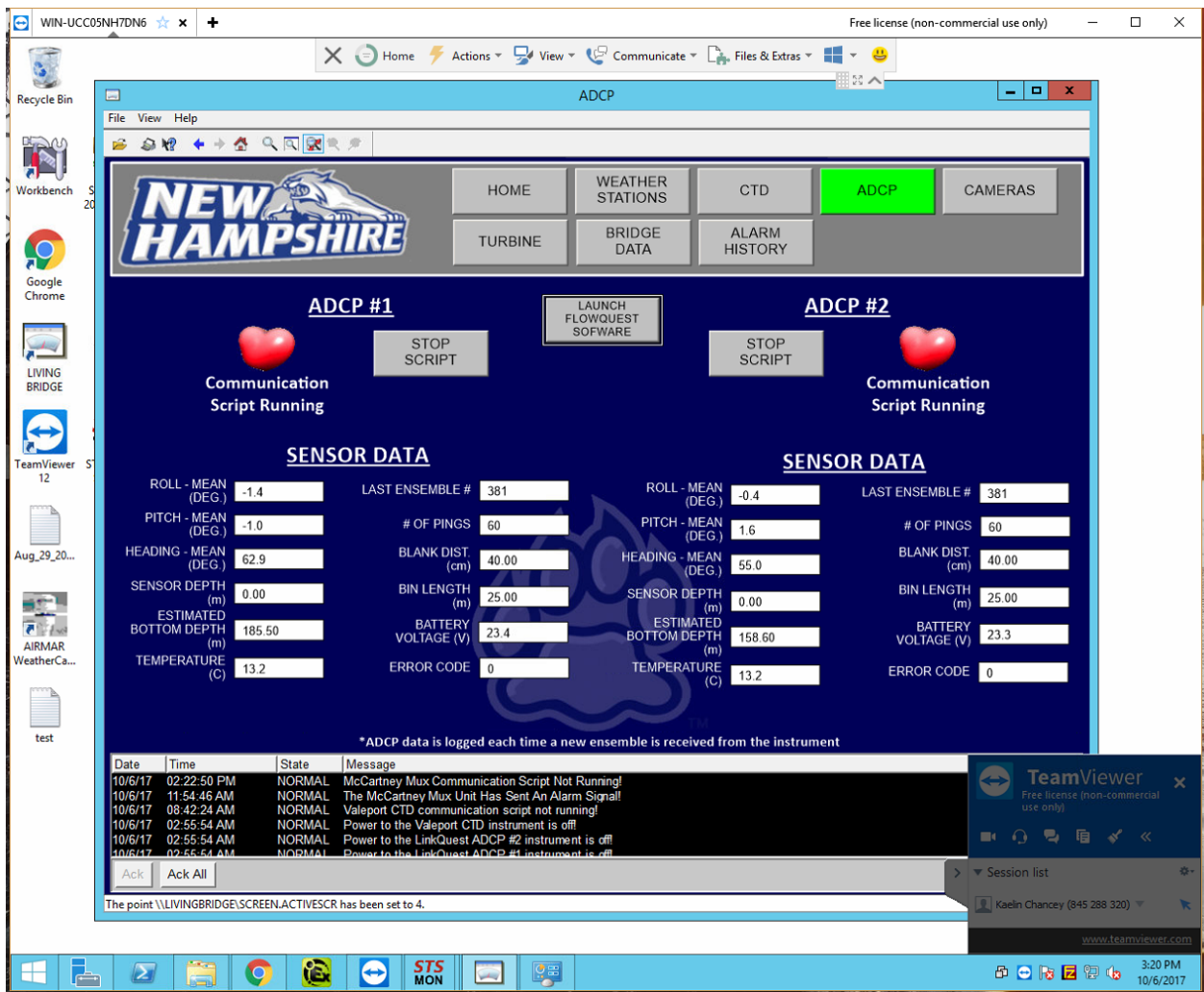
Figure A.4: Living Bridge GUI ADCP page
