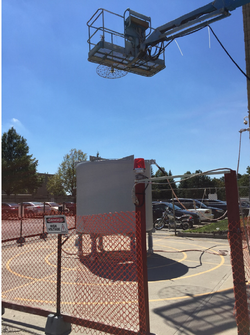
Figure 3-6 – NSI data acquisition top view setup using a Brüel & Kjær 60-channel sector array.
