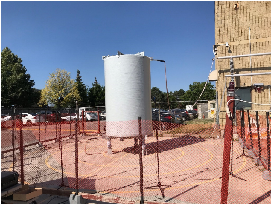
Figure 3-2 – Radial sound measurement experimental test setup for the first prototype reactor.
