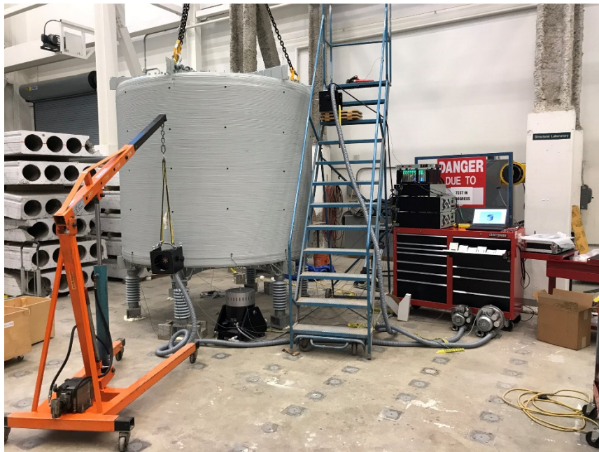
Figure 3-7 – First prototype reactor modal analysis experimental setup.
