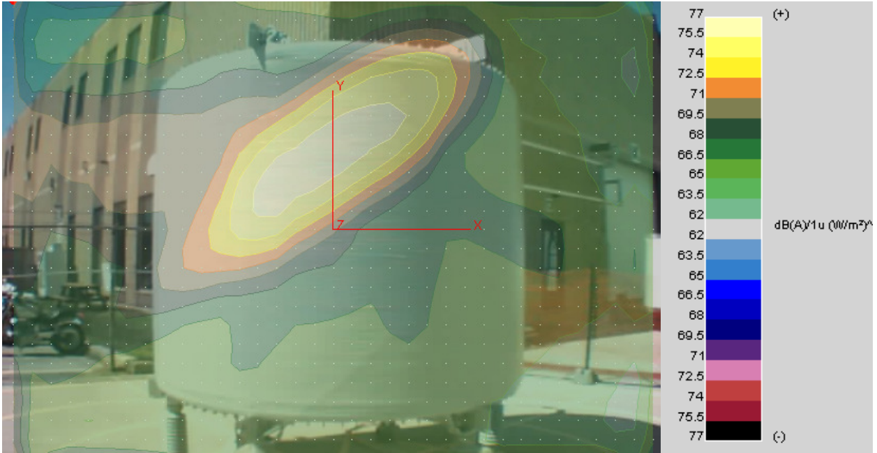
Figure 4-4 – Overall NSI contour plot of reactor sound intensity level energized at 300 Hz - Location 1.
