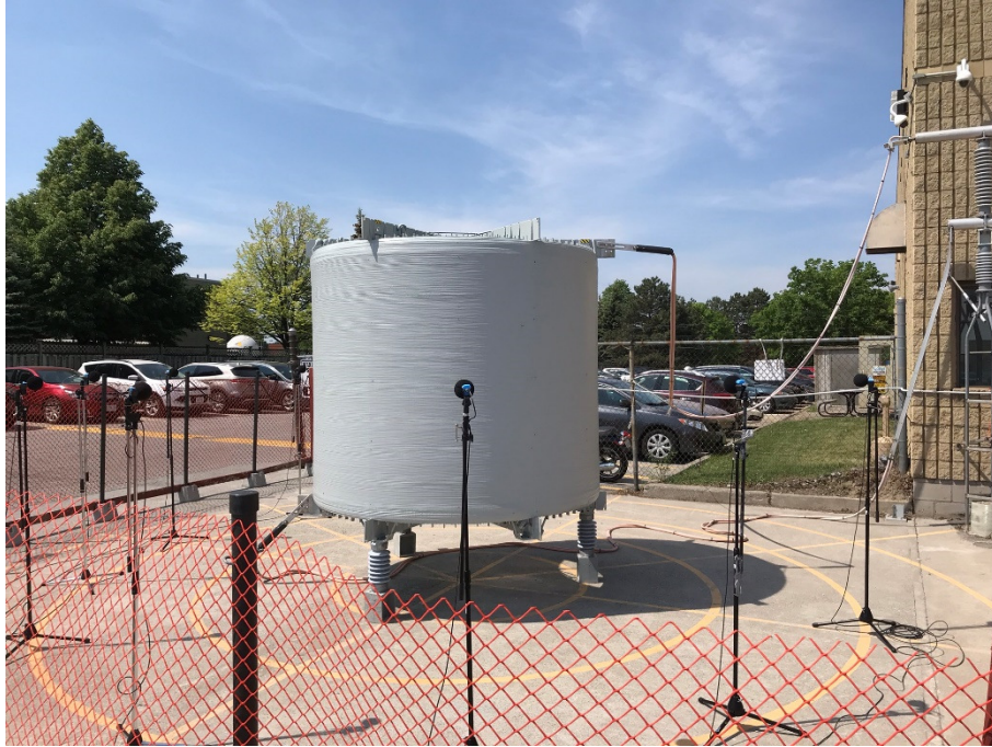
Figure 3-2 – Radial sound measurement experimental test setup for the first prototype reactor.
