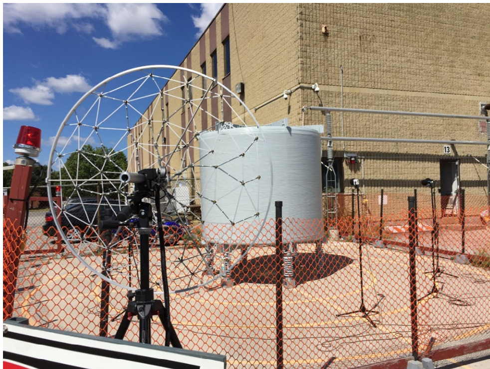
Figure 3-5 – NSI data acquisition setup using a Brüel & Kjær 60-channel sector array.
