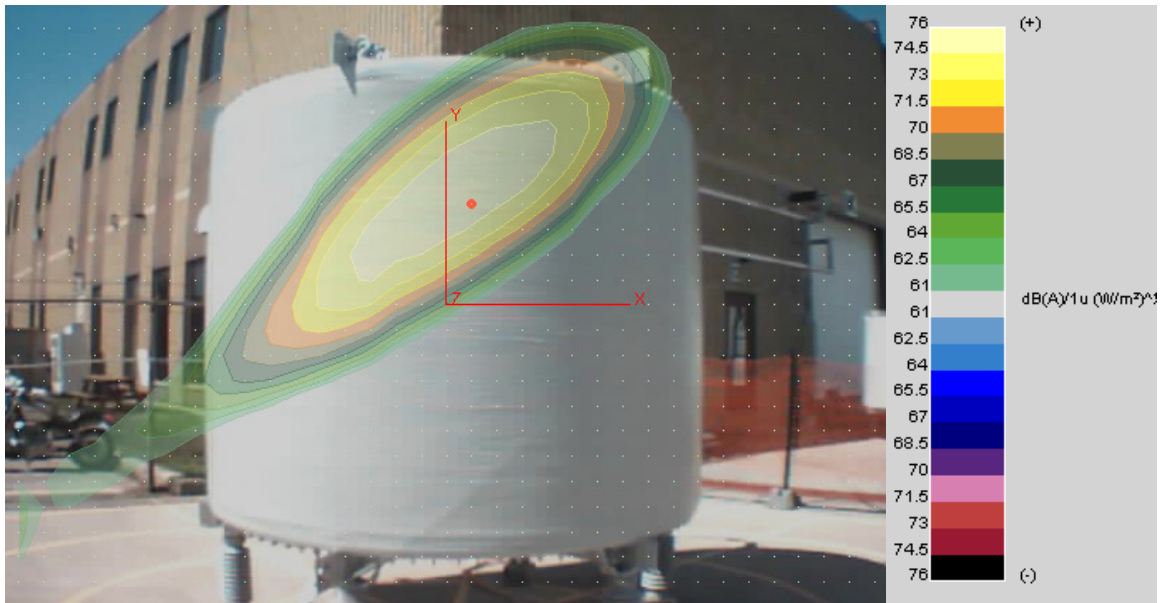
C 1 – 630 Hz NSI contour plot of reactor sound intensity level of reactor 1 energized at 300Hz location 1.
