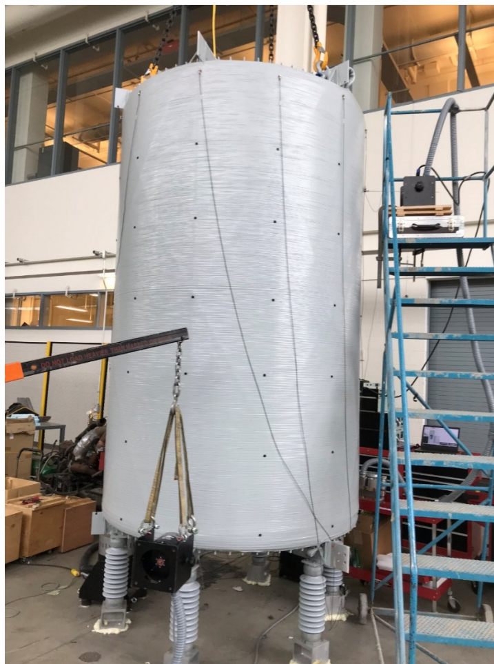
Figure 3-9 – Second prototype reactor modal analysis experimental setup.
