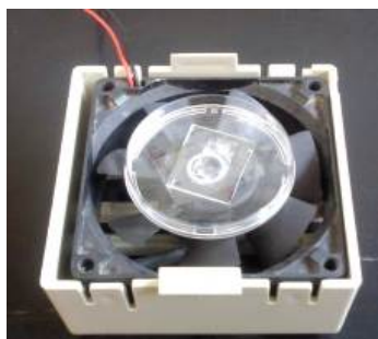
Figure 2. Spin coater/fan set up for AFM sample preparation.
