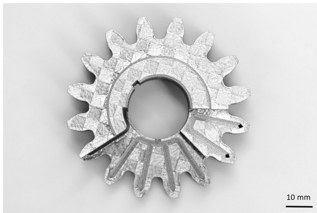
Fig. 6 Gear wheel demonstrator with internal cooling channels manufactured with LPBF
