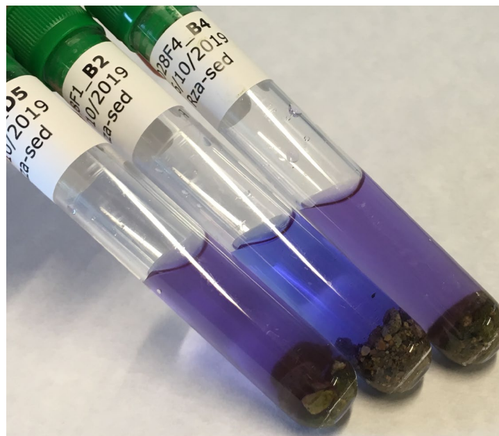
Figure 8: Tubes with sand, tank water and resazurin after four hours of incubation. The purple colour indicates that a reduction to resorufin took place due to aerobic respiration. (Etter, 2019)
