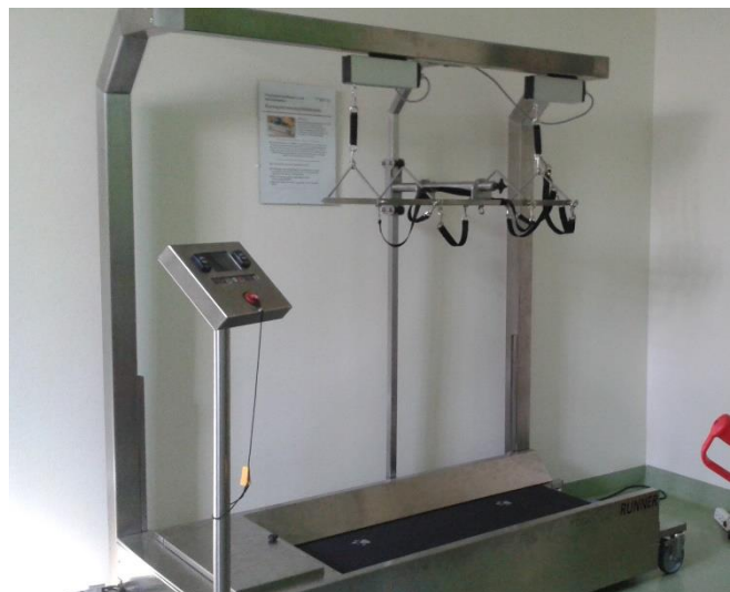
Figure 1 – Treadmill Runner 1™ (Theravet®), equipped with a sling suspension system.
