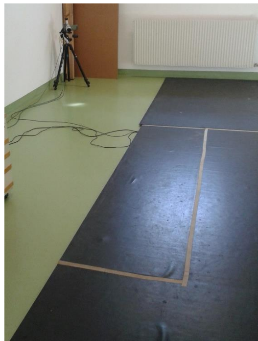
Figure 13 – Pressure plate setting in the motion analysis room. The measurement area is marked with white tape and covered under a rubber mat. In the corner, is the video camera used to film the trials.
