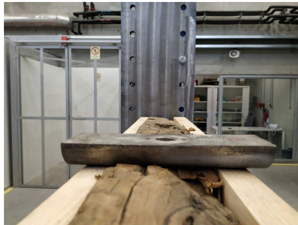
Figure 50 – B-I-G-1: extrados smoothed in order to provide a plain surface for the loading point.
