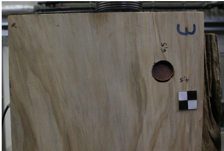
Figure 41 – Failure of sample I-SC-G-1.
