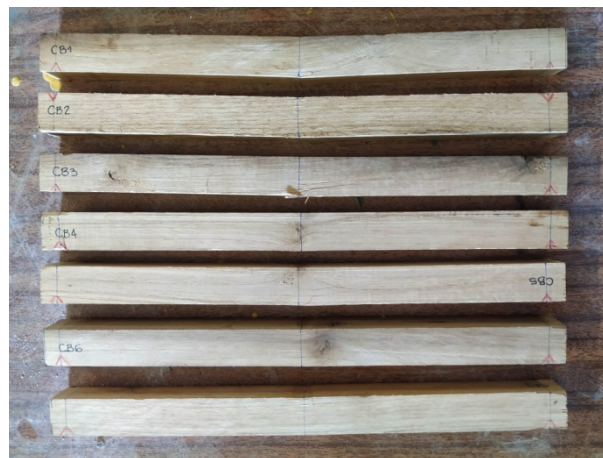
Figure 24 – Failure modes of specimens tested for bending strength.
