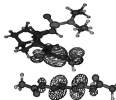
Figure 5. Representation of the LUMO of the dienophile and the HOMO of the diene.
