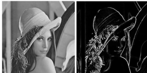
Figure A.0.1 - Convolution layer applied in an image and a resulting feature map [71]
