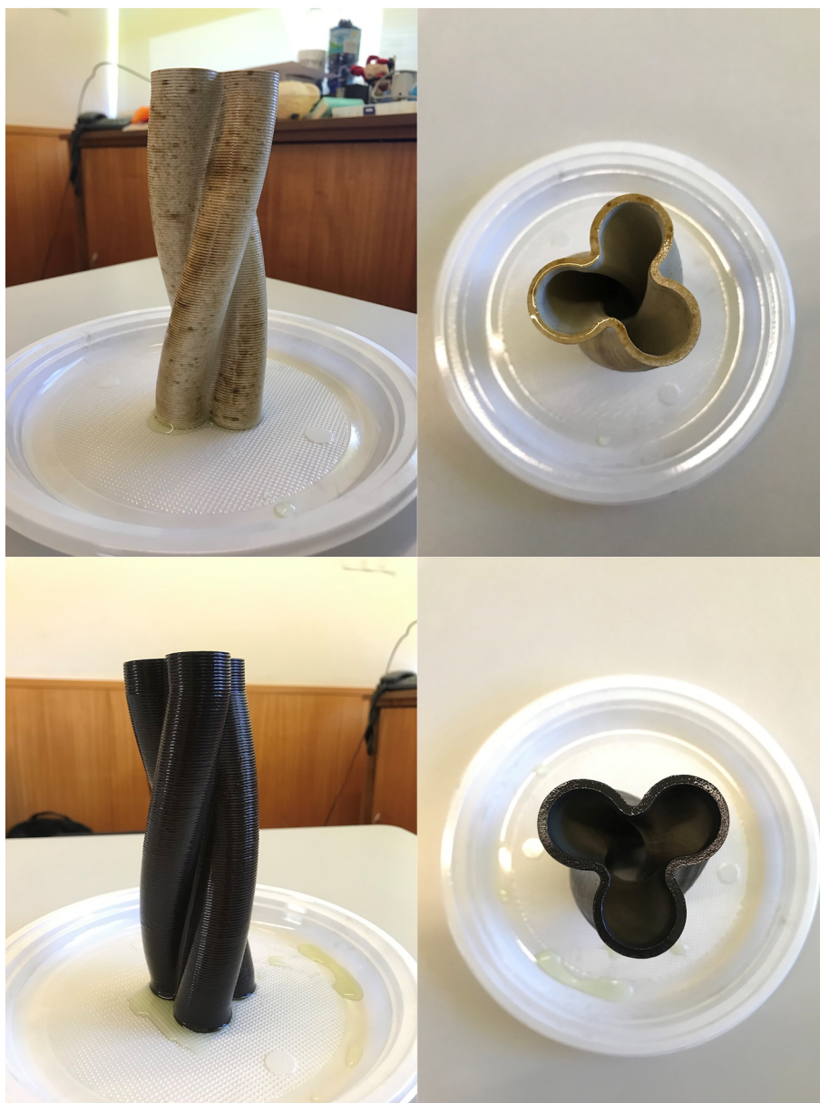
Fig. 9. Functional prototypes in 3D stoneware immersed by 60 days in aquarium water, a) uncoated and b) Ag-TiN coated.
