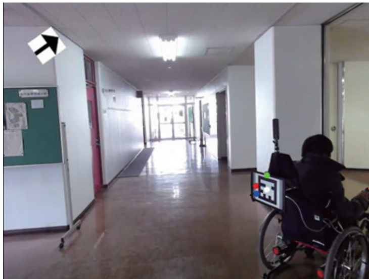
Figure 4.2: System of automatic tracking travel: (a) rear wheelchair utilizes the AR marker to acquire the position of the front wheelchair. By controlling the rear wheelchair according to the position of the AR marker, this research succeeded in following using only the camera, and (b) image of the camera attached to the rear wheelchair.
