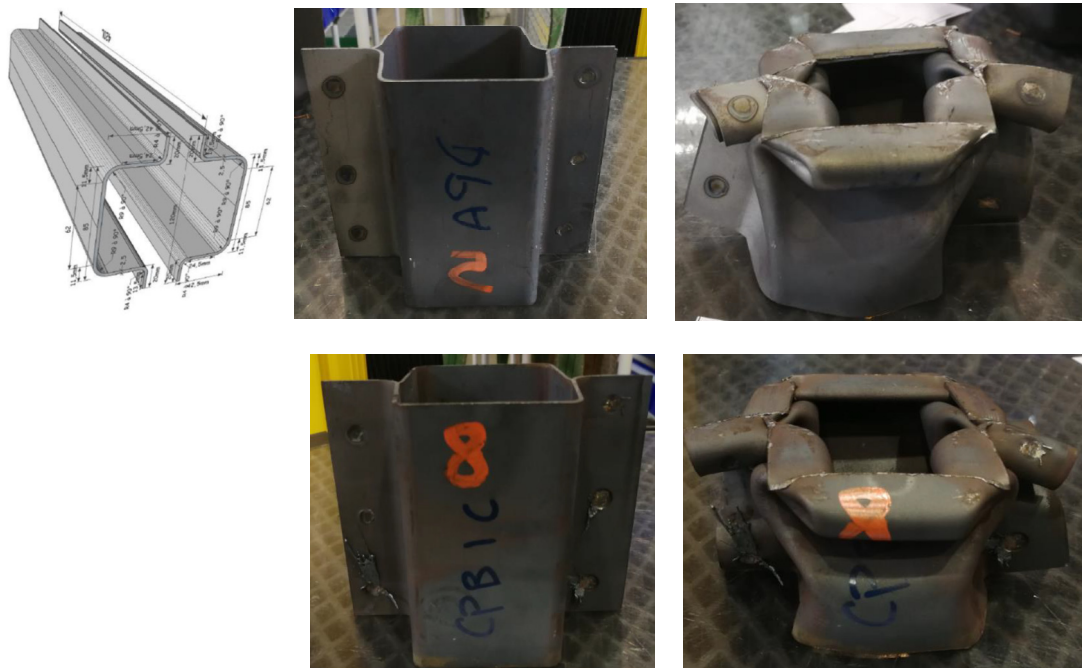
Figure 6: Dimensions and examples of crashed crashcan for DP-A (top) and CP-B (bottom)
