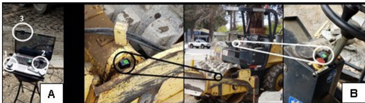
Figure 1. (A) Data Collection Station with the (1) Sensors, (2) Receiver Antenna, and (3) Webcam for Synchronous Video, and (B) Sensor Installation on the Vibratory Roller Body
