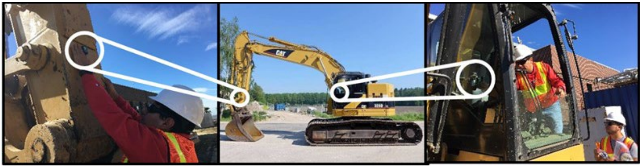
Figure 2. Sensor Installation on Excavator 1 Body
