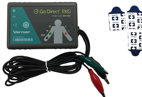
Fig. 4. Single-lead ECG reader and 3 electrodes. Picture taken by the author.
