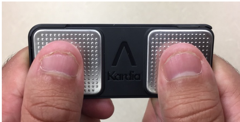
Fig. 6. Single-lead handheld ECG reader. Picture taken by the author.
