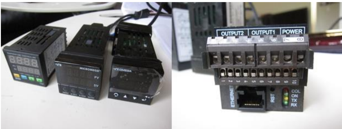
Figure 53. Omega CNi32 PID temperature controller.
