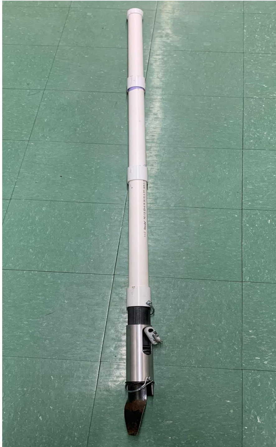
Figure 1.1: The Greenseeder Hand Planter
