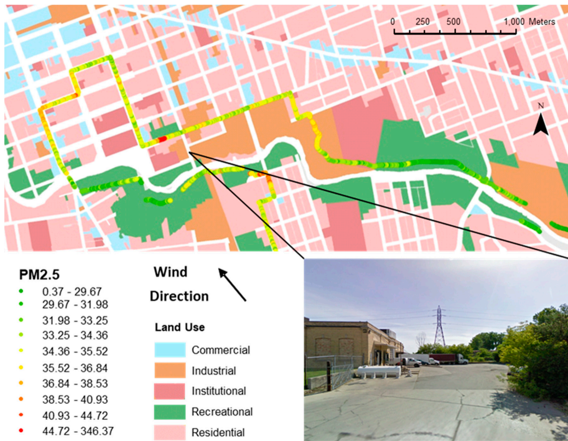
Figure 5. Segment of a single route with 1-s resolution PM_{2.5} concentration measurements overlaid on a land use map. Correlation is apparent between personal exposure to PM_{2.5} and land use. The loading bay with idling vehicles and wind direction may account for the nearby peak in PM_{2.5} concentration in \mu\text{g}/\text{m}^3 .
