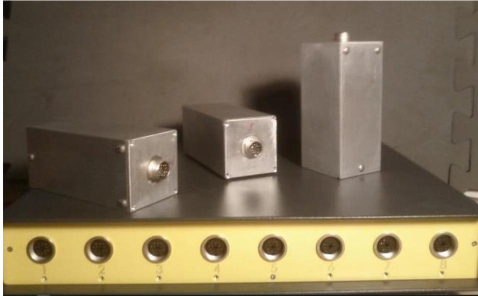
**Figure 4.1: DYNAMate system with 3 DM 4.5 Hz sensors**
