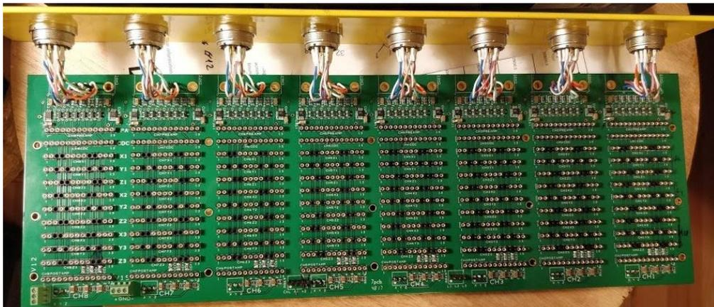
**Figure 4.18: DYNAMate motherboard and back panel plug complete assembly**
