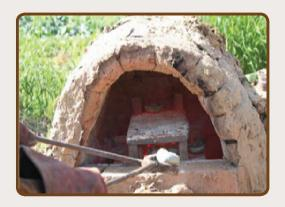
stays inside the kiln. The fire box chamber is then lit and stoked continuously for a designated period depending on how long is required to melt any slips or glazes or any particular special effects desired. We often put pottery temperature cones inside of the pottery chamber of this kiln. Adding a small brick in the pottery chamber entrance that can be pulled out and used as a 'peek' hole allows us to see if the cones have fallen over, thus determining the ripeness of our glazes.
