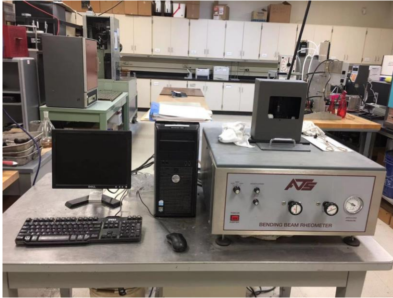
Figure 3.5 the BBR equipment
