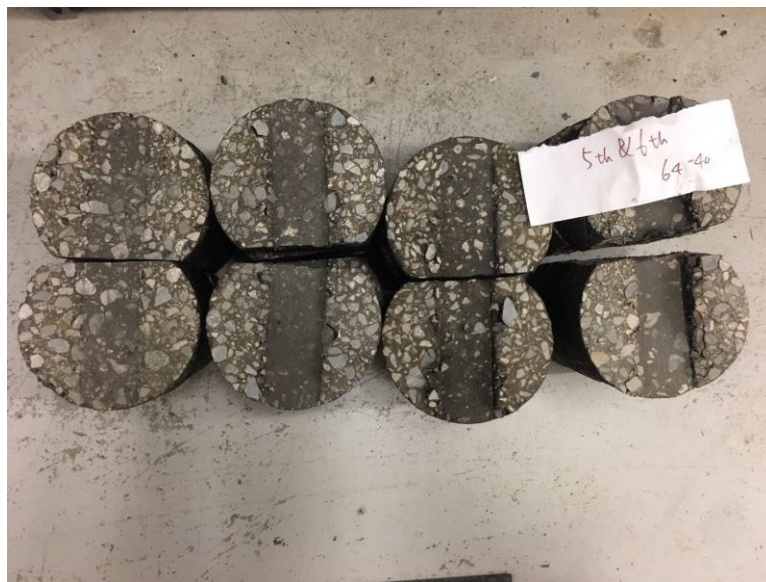
Figure 3.11 HWT specimens after testing
