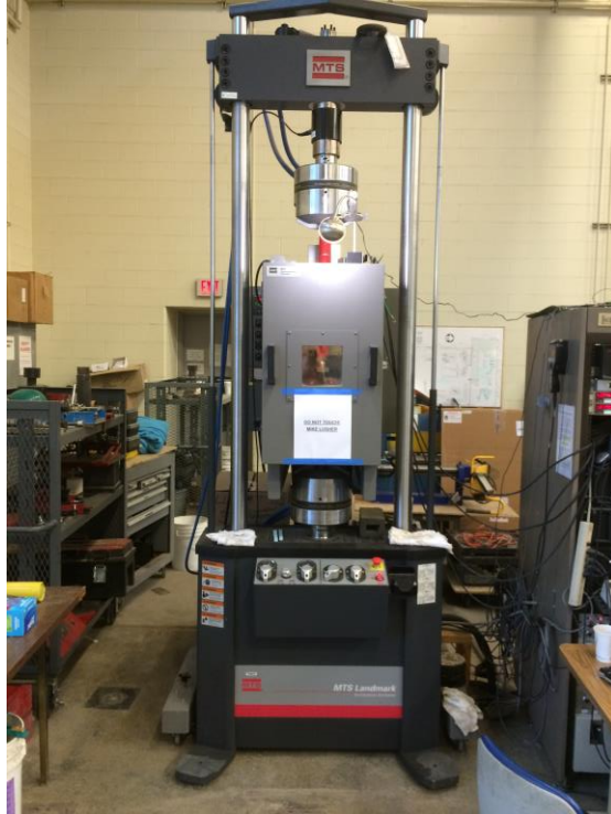
Figure 3.17 IDT test equipment
