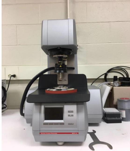
Figure 3.4 the DSR equipment
