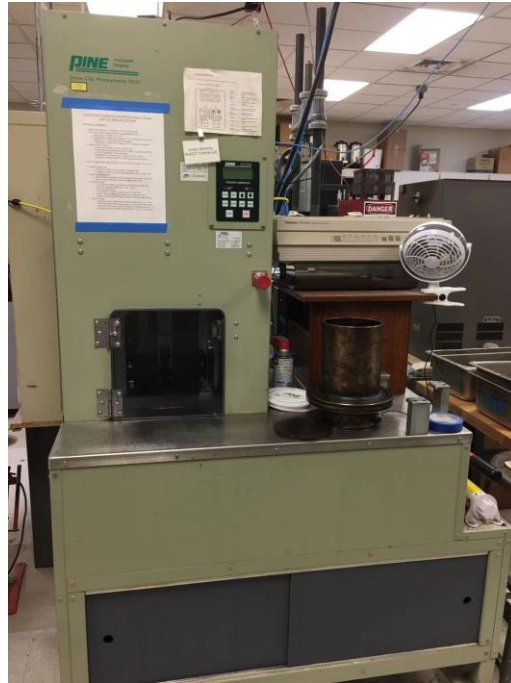
Figure 3.7 Superpave gyratory compactor
