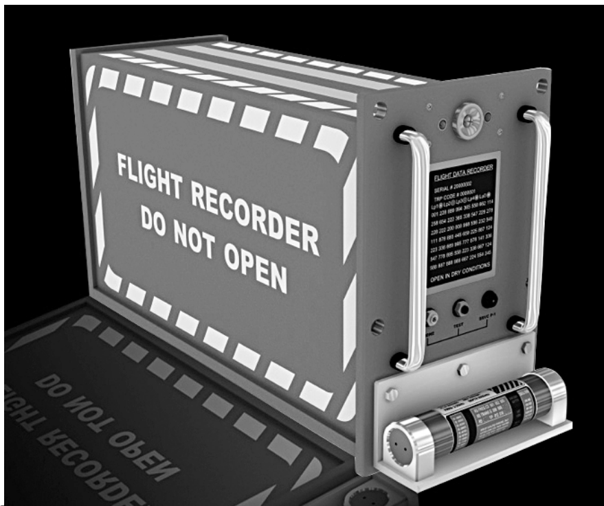
Figure 14: An aeroplane's digital flight-data recorder, or 'black box'
