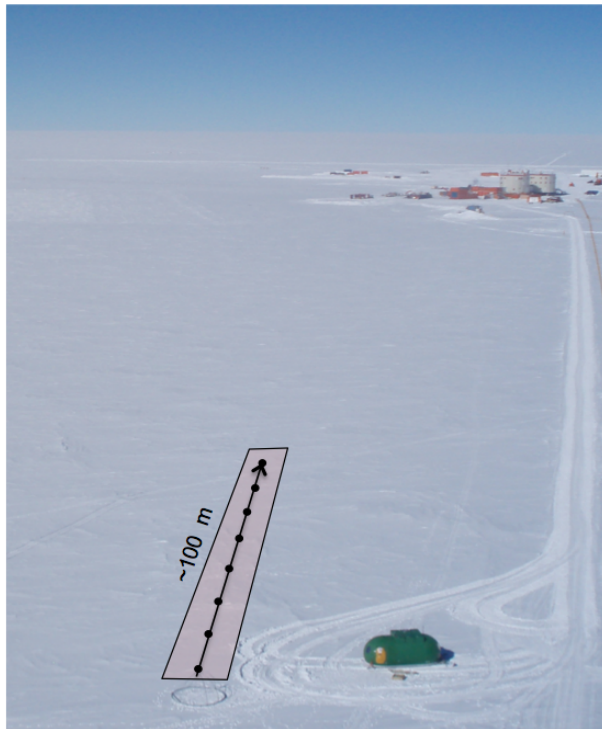
Figure 3: Location of \sim 100 m transect over which GRASS measurements were taken. The transect runs parallel to a little used access “road” running from the main base to the “American tower” from which this photo was taken. The recent disturbed snow was due to tracked vehicles moving GRASS and ancillary equipment into position. To the authors’ knowledge this area has had no anthropogenic ground disturbance for more than a year.
