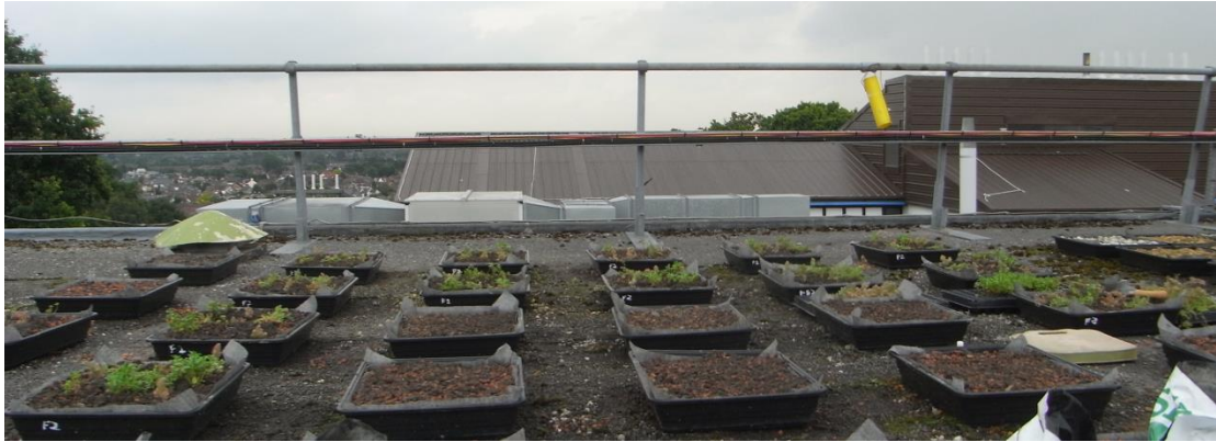
Plate 5.1. New roof at planting. 30 trays were laid out, each with 8cm of crushed red brick substrate.
