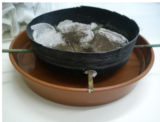
Plate 3.2. Nematode extraction set-up, based on the Baermann funnel technique. The black section comprises of a wide plastic mesh, topped with filter paper. Soil samples are placed on the filter paper and nematodes are collected from the terracotta portion.
