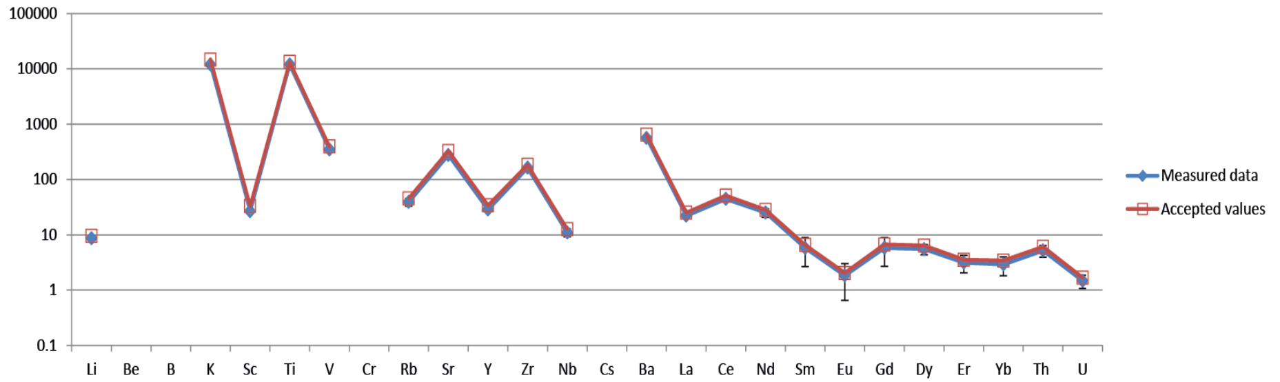
Figure 5.17 comparison of SIMS BCR 2G standard analyses against accepted values. 2SD shown (when larger than symbols) for measured data.
