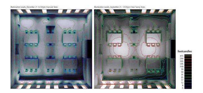
Figure 9. Daylight illumination levels without skylights (left) and with skylights (right). Models by Integral Group, 2018.
