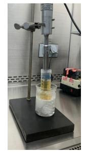
**Figure 6.** Sonication setup under tissue culture hood. The ultrasonic processor head is stabilized by ring stand. LCPAM solution is stabilized by a Styrofoam base and submerged in a beaker of ice.
