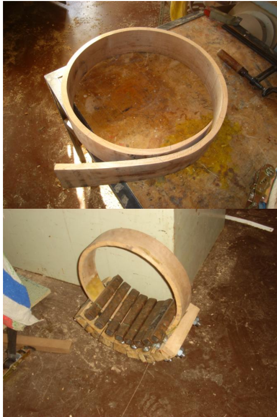
Figure 19: The frame removed from the bending apparatus and gluing the red cherry frame after it had dried for 36 hours.
