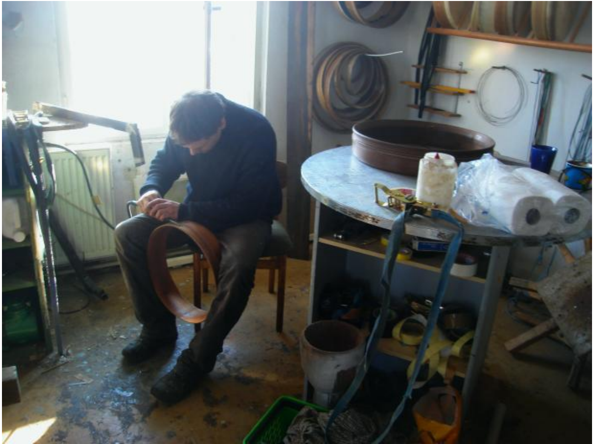
Figure 21: The channel for the inner tube tuning system is being cut into the red cherry frame.
