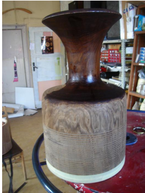
Figure 23: The tonbak after the ammonia "bath" treatment and during the application of linseed oil.
