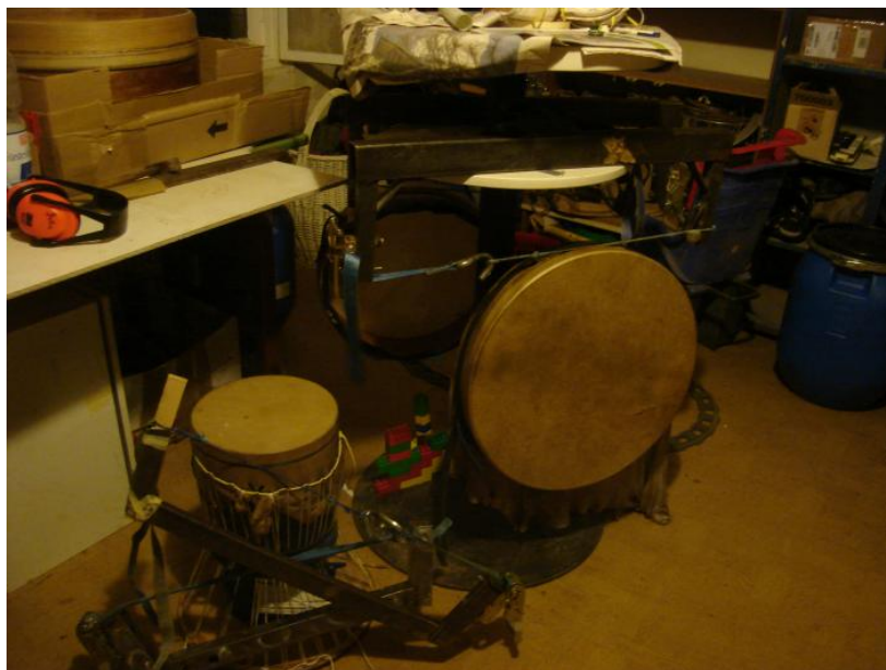
Figure 26: Affixing the skins to the frames and allowing them to dry fully using a tension increasing device to keep them taut.
