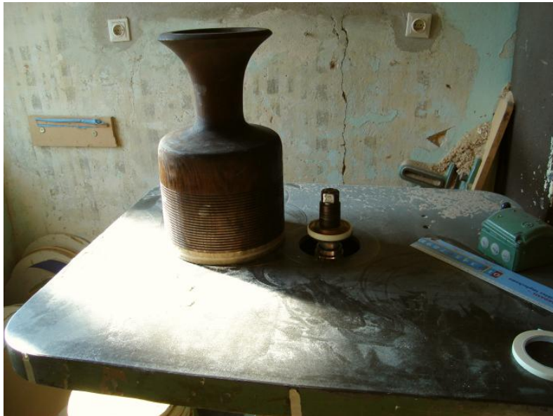
Figure 22: The tonbak after the channels had been cut on the outside of the body.
