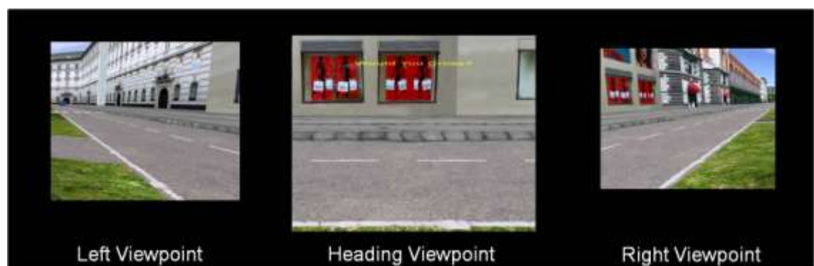
Figure 7.1. Example of experimental set-up testing gap acceptance thresholds in a virtual environment. Six vehicles either approached from the right (one-lane conditions) or from the right and left (two-lane conditions) at 20, 30 and 40 mph.
