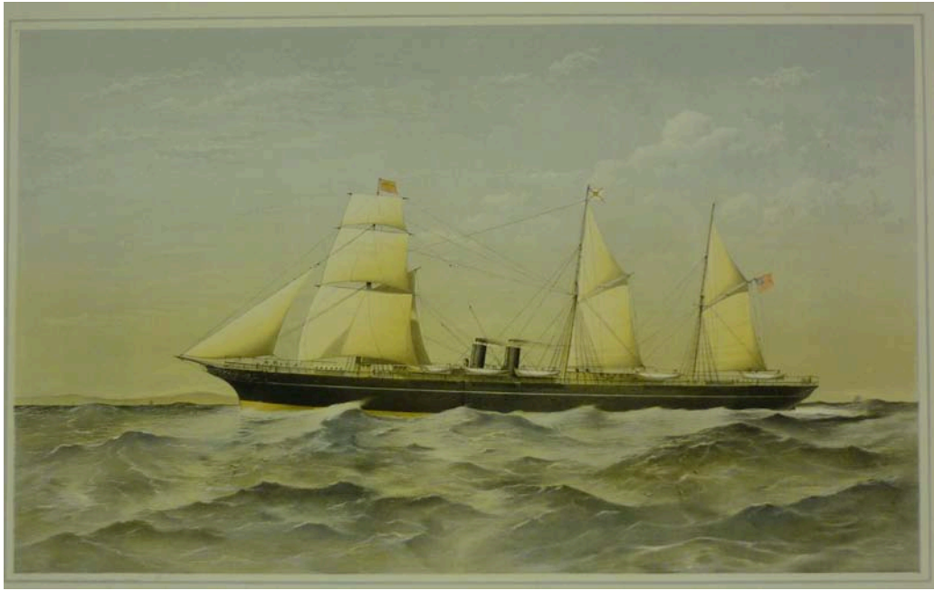
Figure 5.3 The RMSPC's Steam Ship Medway , 3235 tons register, 600 horse power nominal, courtesy of National Maritime Museum, Greenwich, London. The Medway , which entered service in 1877, was a later era steamship with greater passenger capacity and engine power than its predecessors. By the 1880s the RMSPC was constructing vessels to accommodate more than two hundred and fifty first-class passengers, and around thirty second- and third-class passengers respectively. 124
