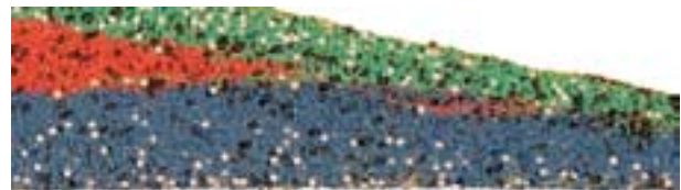
Figure 6.7 Detail of various inverted stratigraphic structures at the distal end of the deposit shown in Figure 6.6B. The left inversion shows green charge 3 material underneath red charge 2 material. The right inversion shows red charge 2 (and a hint of some green charge 3) material underneath blue charge 1 material.
