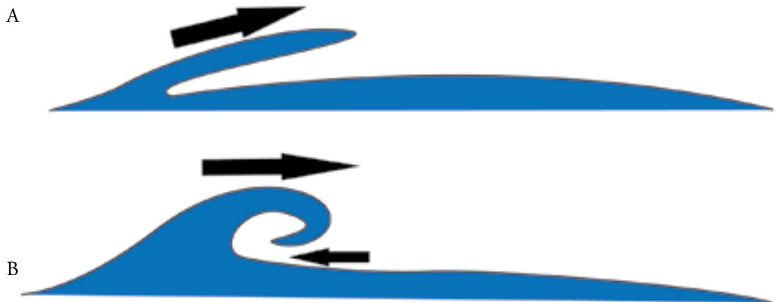
Figure 6.3 Illustration of possible mechanisms for the formation of the reworked structures (A) Loading and shearing of the underlying substrate, and (B) Rotational turnover (i.e. vortex-like).
