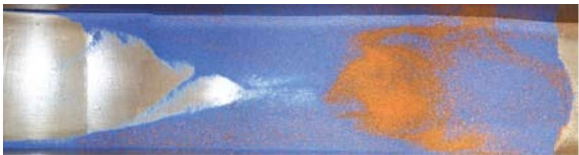
Figure 5.8 Plan view and central section of a 500 cm 3 polymict charge (identical to that in Figure 5.6 and 5.7) run into flume C, large particles in orange.
