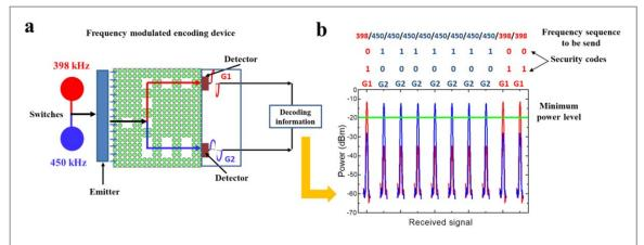
**Figure 6.** (a) Sketch of the acoustic logical device for encoding process with a broadband input pulse with the components of 398 and 450 kHz controlled with intent, (b) demultiplexing is accomplished by spatial modulation of the power output by varying the 398 or 450 kHz frequency components of the pulse. Modulation of the frequency components is achieved through pulse shaping.
