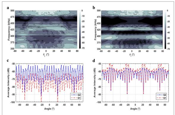
Figure 3. The numerically determined quasi-density of states for the upper G1 (a) and lower (b) channel G2 of the forked CRAW device. Transmission intensity was measured at the output for each channel for incident angles ranging from  $+90^{\circ}$  to  $-90^{\circ}$  with darker shading corresponding to decreased transmission. The defect modes of 450 (c) and 398 kHz (d) express varying mode coupling strength between channels.
