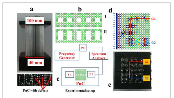
$\begin{tabular}{l} Figure 1. (a) Optical picture of the phononic crystal (PnC) (above) and its corresponding defect line (below). (b) Sketches of the coupled-resonator defect cavities (Models I and II). (c) Experimental set up used for measuring transmission spectra. (d) Field of propagating sound in the two channels (G1, G2) of the coupled resonant acoustic waveguide (CRAW) using COMSOL with its corresponding optical images in (e). \\ \end{tabular}$
