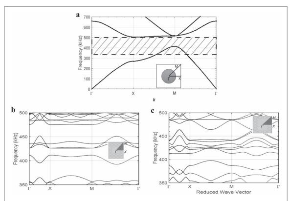
**Figure 2.** (a) Band diagram of the lattice of the CRAW device without defects. The structure is examined from 350 to 500 kHz indicated by dashed square. Inside the gap, the band diagram is given for a Model I (b) and Model II (c) defect using the superlattice approach. The defects open up different allowed modes as shown by their bandstructures.
