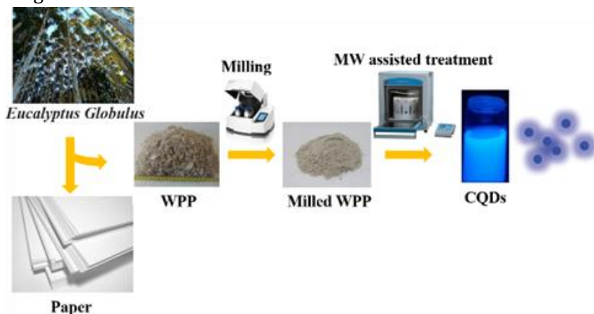
Figure 1. Schematic approach to obtain CQDs from WPP.
