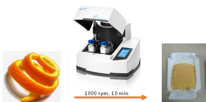
Figure S1. Schematic representation of orange peel pre-treatment.
