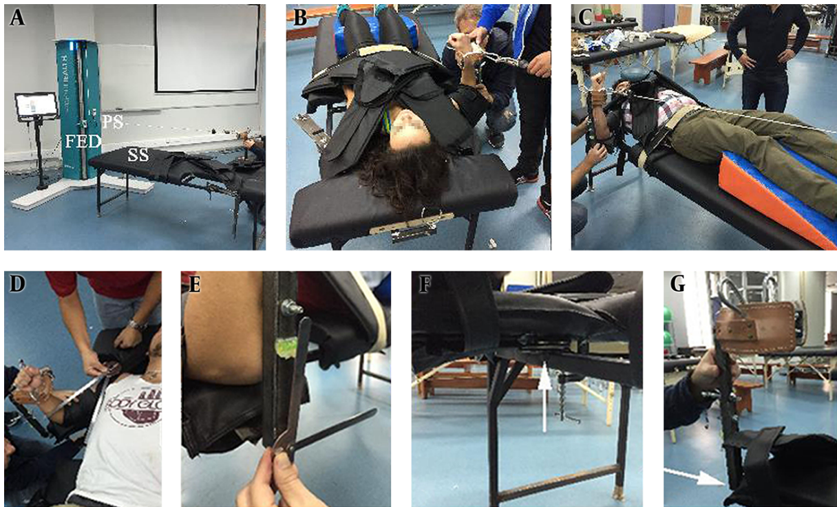
Figure 2. Strength testing for shoulder rotators. A, Experimental setup (FED = electromechanical dynamometer, PS = pulley system, and SS = stabilizer system). B, Assessment position. C, Rigid attachment at 90° angle. D, Shoulder goniometry assessment. E, Forearm orientation. F, Proximal joint of the stabilizer system: white arrow shows the joint axis. G, Distal hinge joint of the stabilizer system: white arrow shows joint axis.
