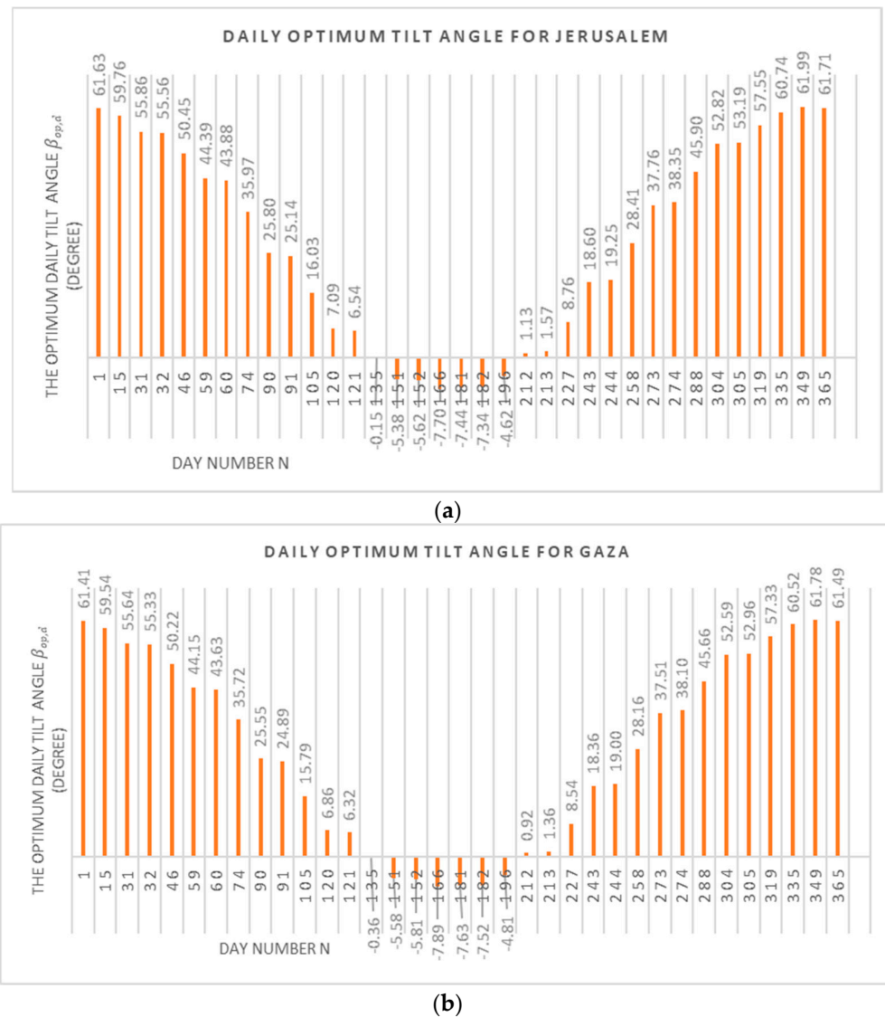
Figure 4. The daily optimum tilt angle \beta_{opt,d} for Jerusalem (a) and Gaza City (b).
