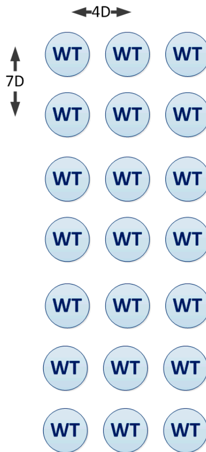
Figure 1. Distance between offshore wind turbines (4D) and distance between lines of offshore wind turbines (7D).
