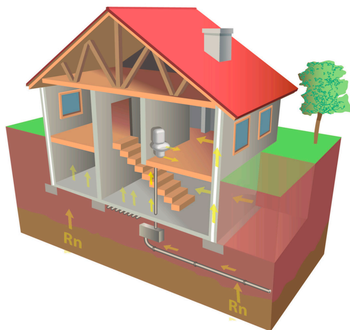
Figure 2. Radon accesses to a home: access through cracks in the subsoil, accumulation in lower floors and/or basements due to poor ventilation, through water pipes that are contaminated in the subsoil and transfer radon to higher levels, where it is filtered through taps, toilets and/or showers.
