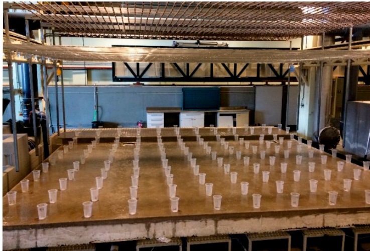
Figure 3. Vessels disposed over the entire model surface in a 0.5 m × 0.5 m grid to measure rain intensity and uniformity.
