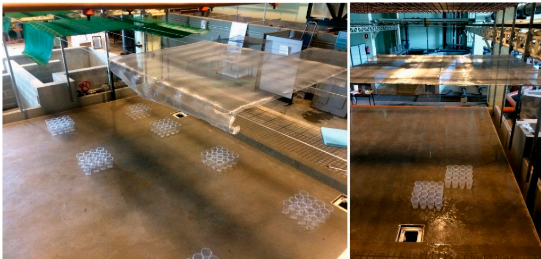
Figure 2. Vessels disposed over the model surface to measure rain intensity and uniformity for different mesh types and distances to drippers during calibration.
