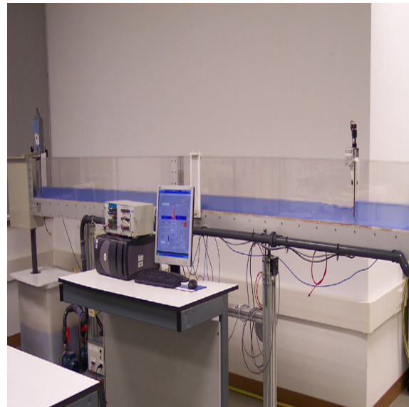
Figure 1: Prototype hydraulic canal in laboratory
