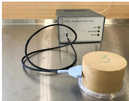
**Figure 3.4-** Measurement of thermal conductivity with the hot wire method
