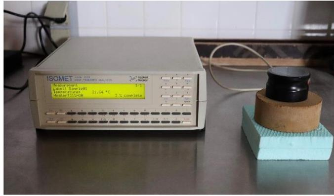
**Figure 3.3-** Thermal conductivity test using the contact probe method
