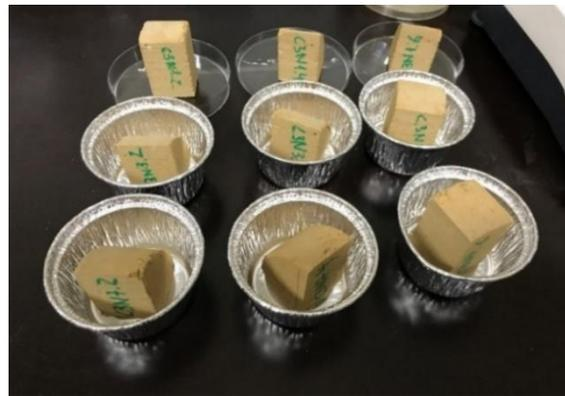
**Figure 3.9-** Example of samples used for the sorption isotherms determination
