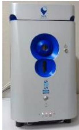
**Figure 3.11** – Dynamic Vapour Sorption equipment (Intrinsic 2, SMS®)
