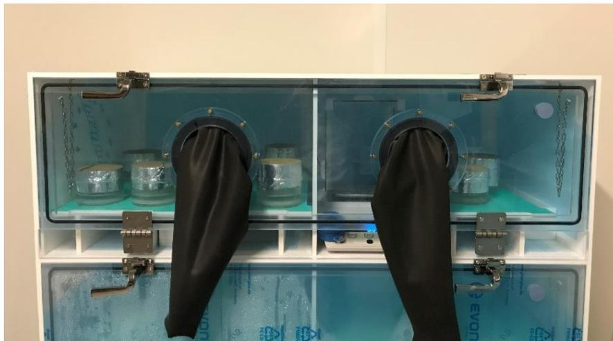
**Figure 3.8-** Wet cup test setup performed in gloves box
