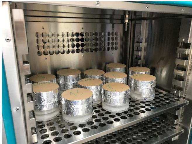
**Figure 3.7-** Wet cup test setup performed in climatic chamber
