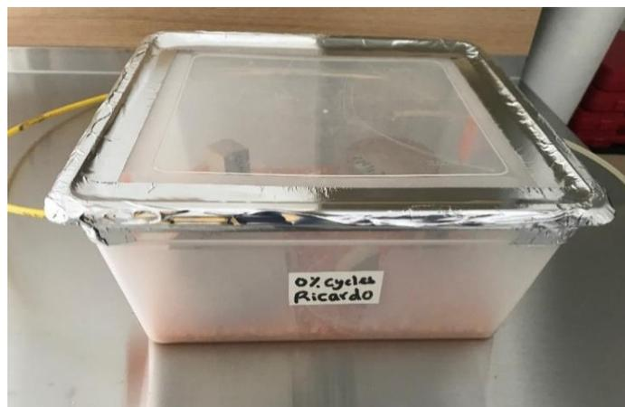
**Figure 3.13-** Samples placed in plastic box with dry air flow for drying at 0%
