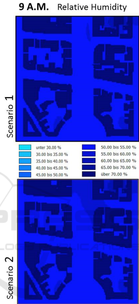
Figure 10: Relative Humidity in Scenario 1 and Scenario 2 simulated in ENVI-met at 9 A.M.
