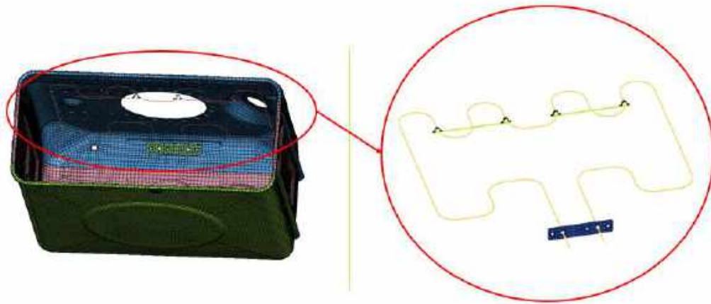
Figure 3-12. Upper heating grate location.
