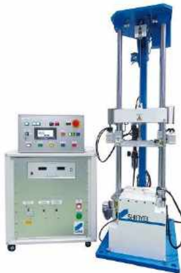
Figure 2-4. Dynamic compression tester. Source: Shinyei Testing Machinery CO., LTD.
