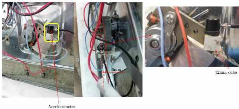
Figure 4-10. Correct positioning of the accelerometer on the Hot Air Motor's physical component. Source: Electrolux
