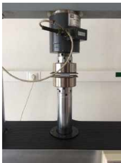
Figure 3-26. First test specimen after compression.
