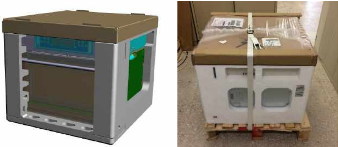
Figure 3-1. a) Geometric model of the oven with packaging. b) Physical model of the oven with packaging.
