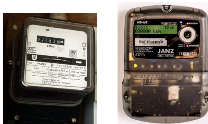
Figure 2.2: Traditional and Smart Electricity Meters.
