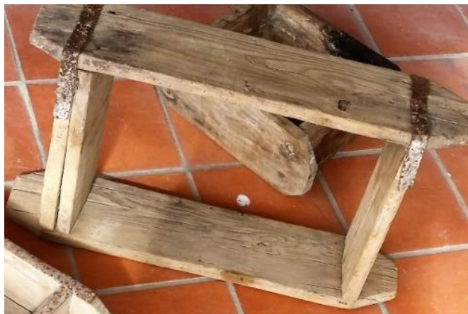
Figure 2. Wooden mold used for vernacular adobe production
