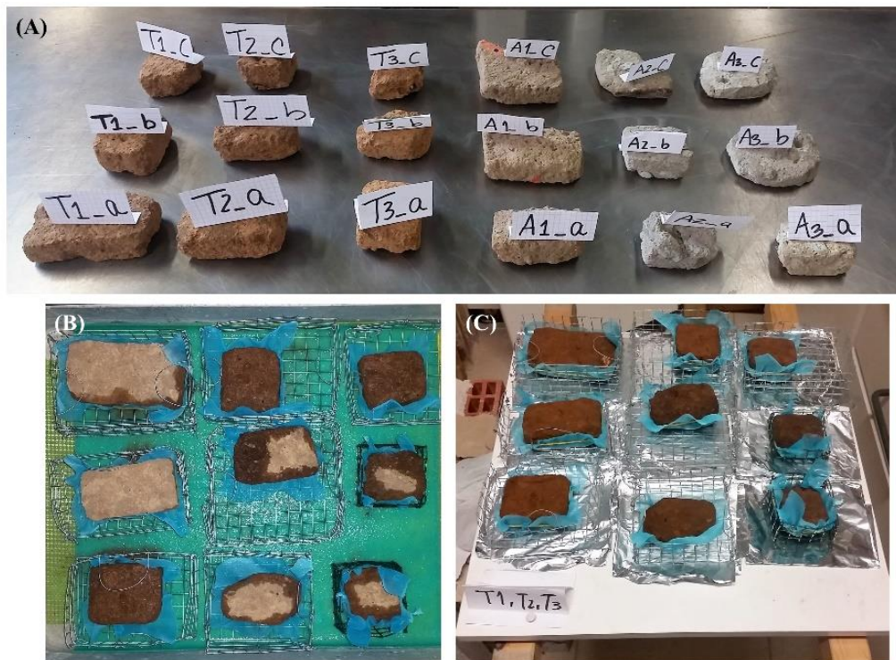
Figure 5. Samples of smaller dimensions (SSD) before the capillary absorption test (A); some samples during the capillarity test (B) and the drying test (C)
