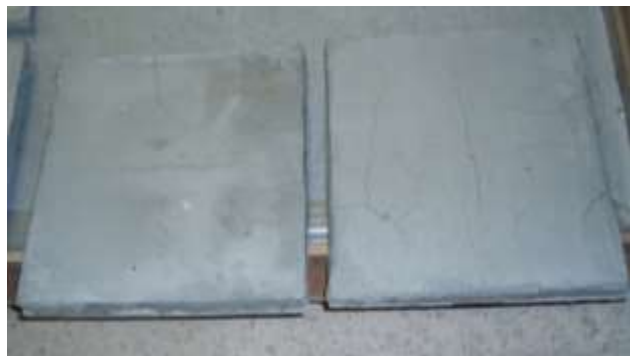
Figure 1 – Restrained shrinkage tests: a) Uniaxial test; b) Slab test
