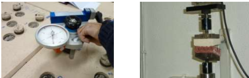
Figure 2 Adhesion with a) pull-off apparatus and b) tensile machine
